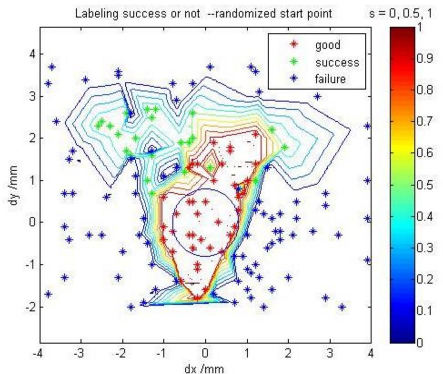
Figure 2: Uniform distributed noise added to the robot to get the acceptable error for start point. It shows that the acceptable error to satisfy the task for start point is 0.8 mm.
