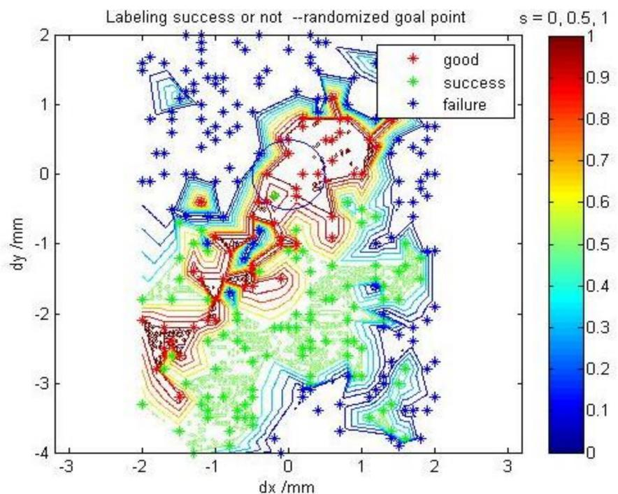
Figure 3: Uniform distributed noise added to the robot to get the acceptable error for goal point. It shows that the acceptable error to satisfy the task for goal point is 0.5 mm.
