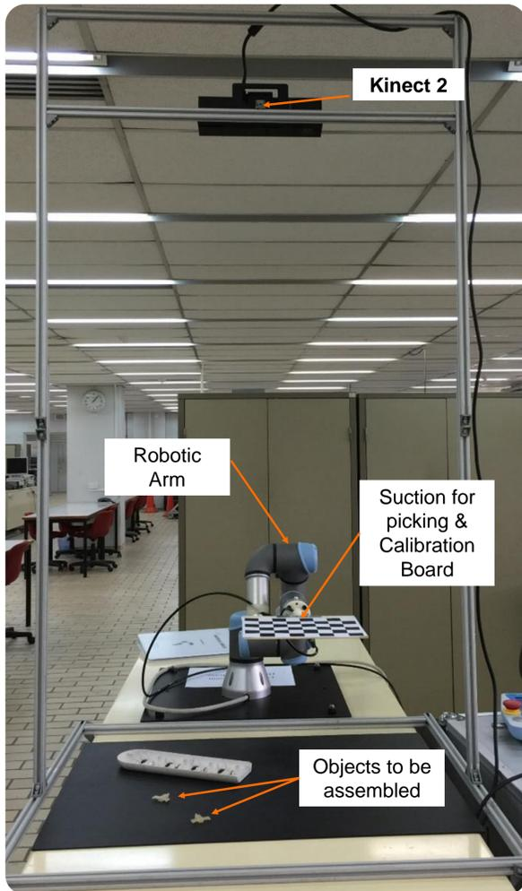
Figure 1: Experimental setups, which consist of a Manipulator with a pneumatic end effector, and a Kinect 2.
